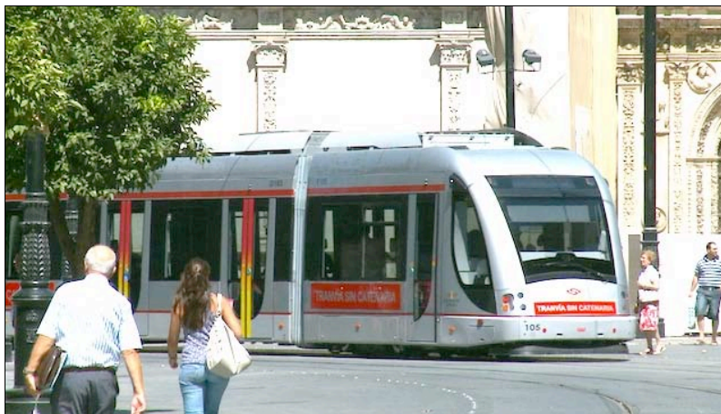
Figure 35: CAF Catenary-free streetcar (Photo Courtesy of Trainelec)
